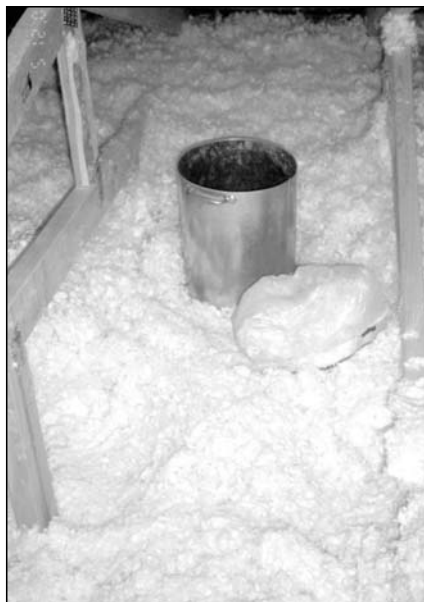
A core sample or cookie-cutter test involves taking at least three insulation samples and weighing them.
