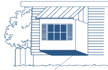
Figure 19: Insulate under bay windows with insulation blankets, batts, rigid foam board or spray-in-foam.
