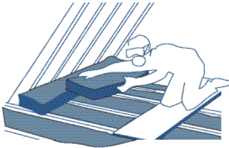
Figure 9: Insulation may be layered over and at right angles to the joists.
